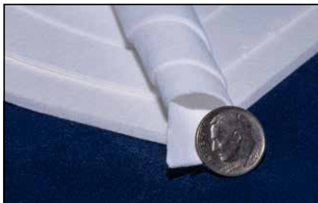
The dime for scale shows the wrappability of ZYF-50 and thickness of ZYF products.
